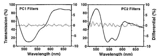
Fig. 3. Transmissions of PC1 and PC2 filters. Solid curves, designed optical filters; dotted curves, calculated filters; dashed curves (barely perceptible), differential transmissions between optical and calculated filters.
